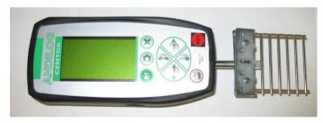
Grid or wire for the grip strength measurements (specifically designed grids (grids only!) are sold by PanLab for 350€, however can easily be assembled from materials which can be purchased from a local do-it-yourself store)
