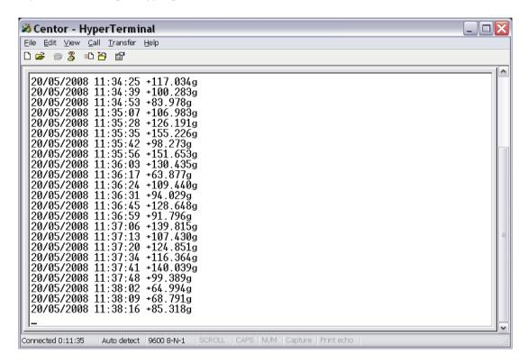
Screenshot of the data as can be seen, if the data are transferred from the Centor Easy force meter to the HyperTerminal program. Similar data sheet can be obtained with other software for data acquisition.
