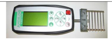
Grid or wire for the grip strength measurements (specifically designed grids (grids only!) are sold by PanLab for 350€, however can easily be assembled from materials which can be purchased from a local do-it-yourself store)
