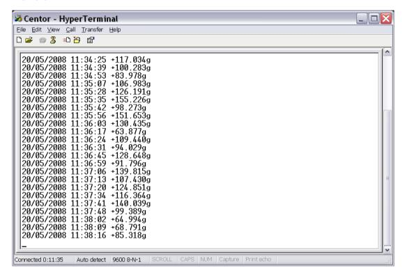
Screenshot of the data as can be seen, if the data are transferred from the Centor Easy force meter to the HyperTerminal program. Similar data sheet can be obtained with other software for data acquisition.
